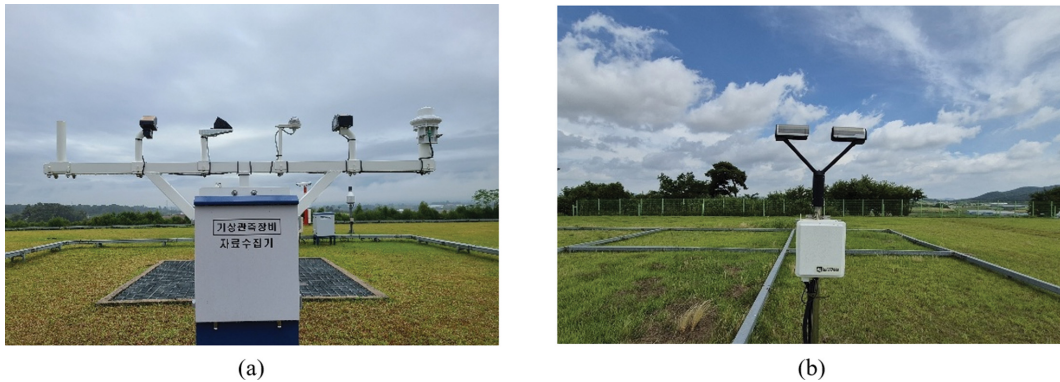
Fig. 2. (a) Comparative observation of rain detectors, (b) Optical disdrometer (Parsivel 2 ).
