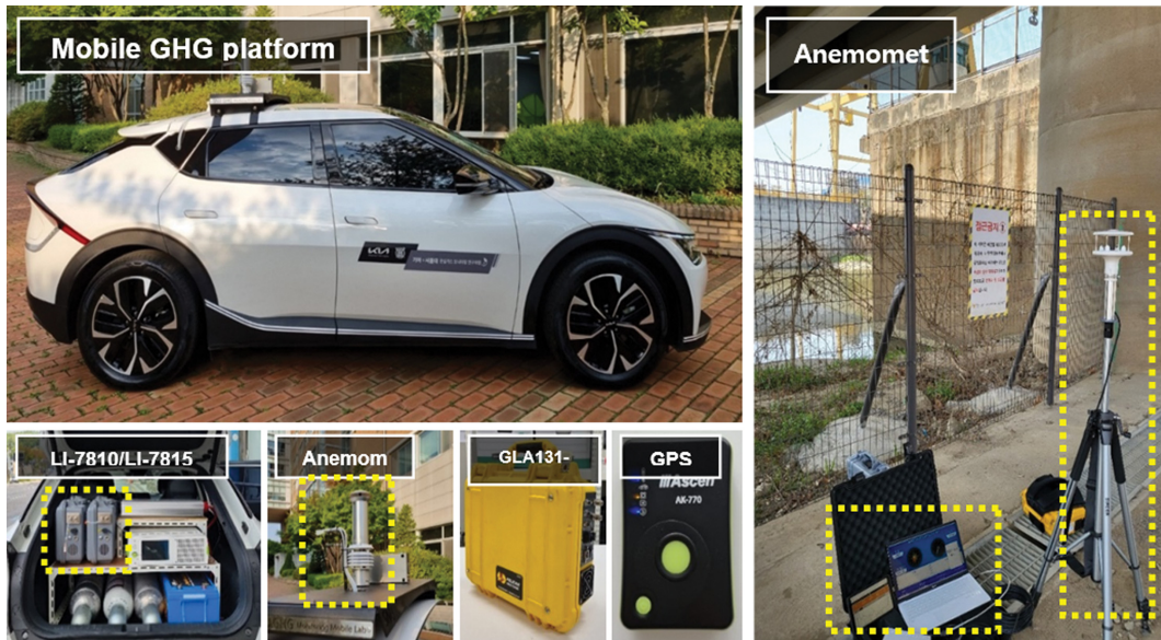
Fig. 1. Vehicle-mounted mobile GHG platform: analyzer rack with LI-7810/LI-7815 fast-response analyzers ( \text{CH}_4/\text{CO}_2/\text{H}_2\text{O} ) and calibration cylinders; portable anemometer mast for on-site meteorology; ABB LGR GLA131-MEA analyzer for \text{CH}_4/\text{C}_2\text{H}_6 source attribution; high-precision GPS/GNSS receiver for position/time synchronization; and a field laptop/logger with power unit for data acquisition.
