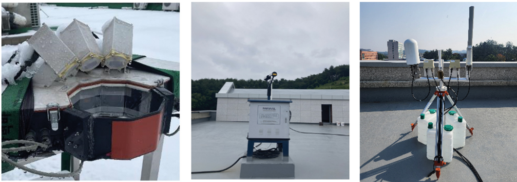
Fig. 2. Pictures of MASC (Multi-Angle Snowflake Camera), PARSIVEL (PARticle SIze and VELOCITY), and radiosonde used in this study.
