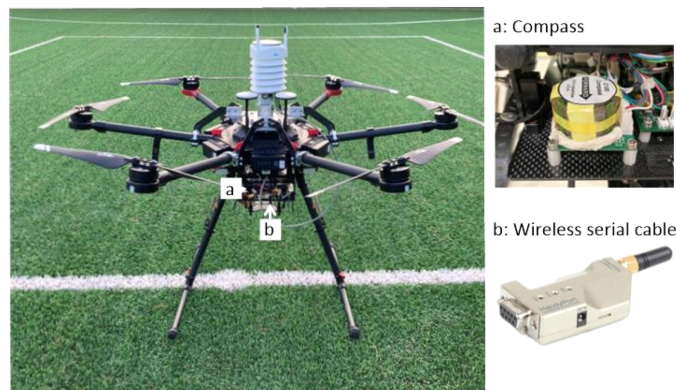
Fig. 3. A drone (Matrice 600 pro) equipped with a meteorological sensor (WXT536). 'a' is compass to calibrate wind direction and 'b' is wireless serial cable to transmit data.
