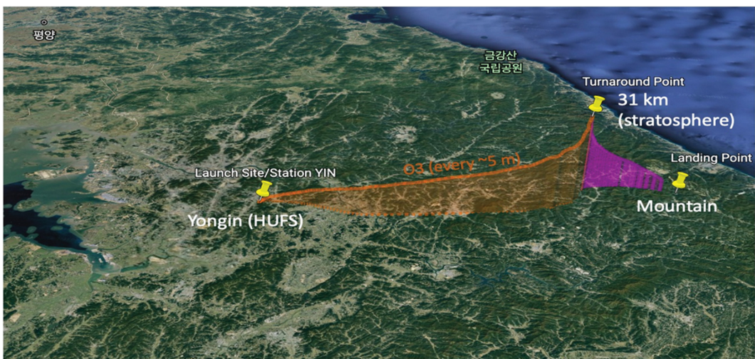
Fig. 3. An example showing the horizontal movement of ozonesonde during measurement.
