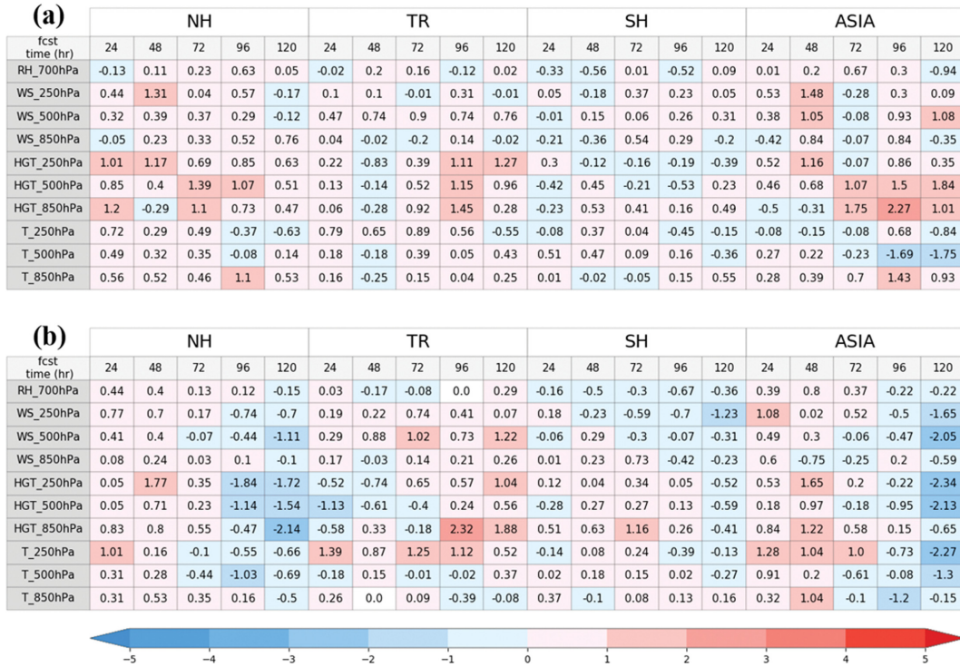
Fig. 9. Improvement rate of RMSD of EXP of analysis against CTL over NH, TR, SH, and ASIA for (a) 0000 UTC and (b) 1200 UTC. Red color means that EXP shows better forecast performance than CTL.
