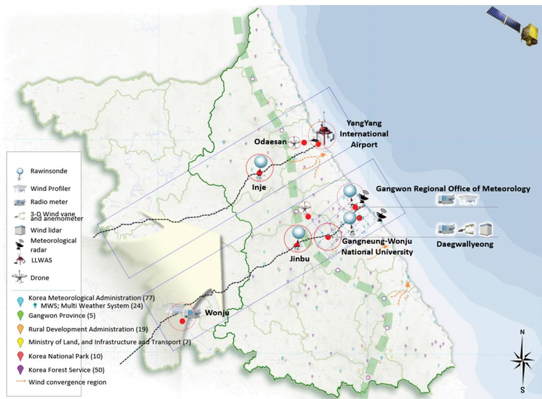
**Fig. 1.** Network of the observing sites in Gangneung and Daegwallyeong region reporting measurement data during G-WEX.
