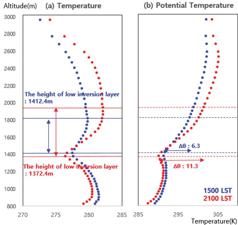
**Fig. 6.** (a) Temperature (b) Potential Temperature of Radio meter at Daegwallyeong during IOP 5: red line for 1500 LST and blue line for 2100 LST on 28 April.
