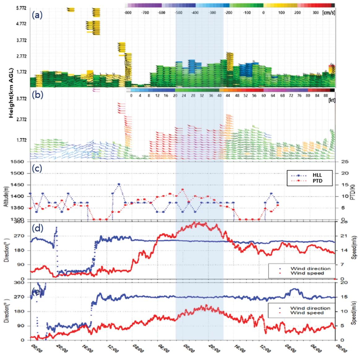
**Fig. 5.** (a) Vertical wind velocity and (b) horizontal wind velocity of Wind Lidar at Daegwallyeong, (c) height of the low level in the inversion layer and its potential temperature difference, and (d), (e) AWS wind direction & speed at Seonjaryeong and Daegwallyeong.
