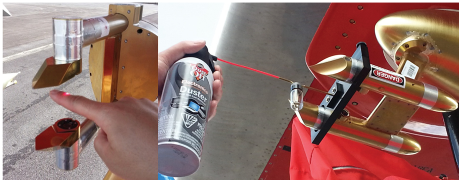
Fig. 2. Pictures of a cloud imaging probe (CIP, left) and a cloud droplet probe (CDP, right). The CIP laser is illuminating on a finger near the sample area of CIP. An air spray with a calibration tool kit (black plastic plate) are also shown with the CDP.
