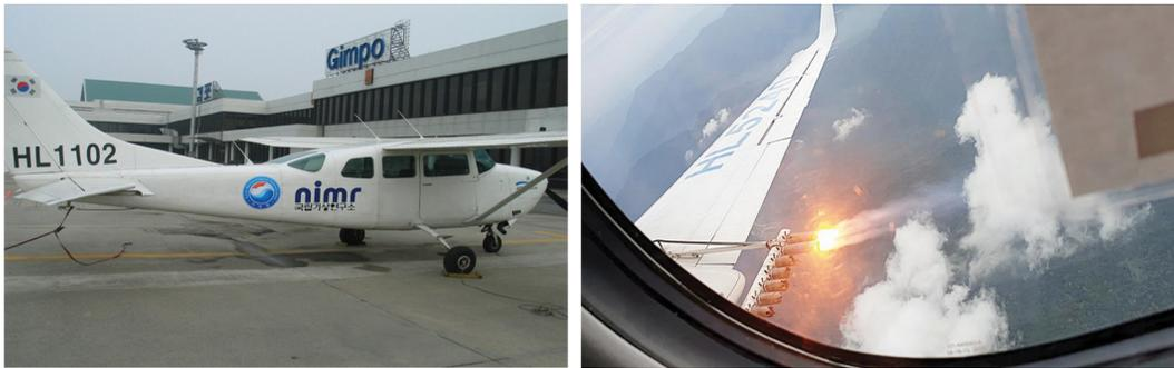
Fig. 1. Images of leased aircraft (CESSNA-206) (left) and Burn-in-place cloud seeding flare (Right).
