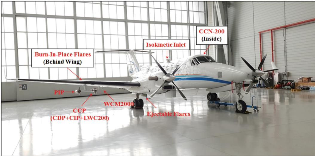
Fig. 2. Atmospheric research aircraft and cloud observational instruments of NIMS.
