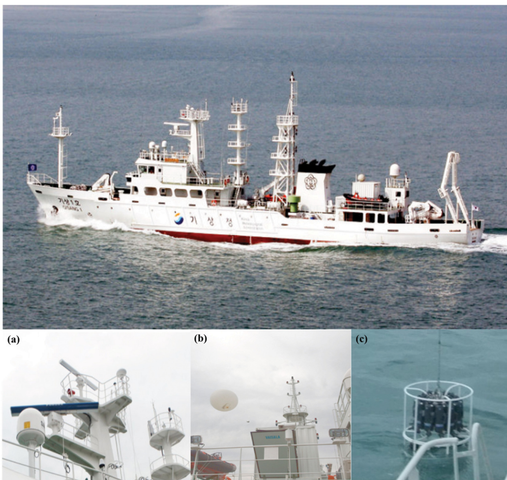
Fig. 4. The KMA research vessel (Gisang 1) operating (a) ocean meteorological observation, (b) upper level meteorological observation, and (c) ocean observation.
