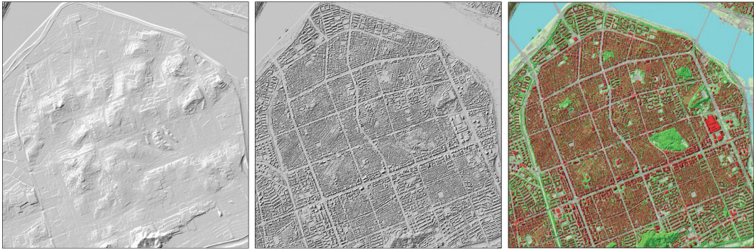
Fig. 2. Three spatial information data (DTM, DSM, and LC) of the CAS simulation around the Seonjeongneung region.
